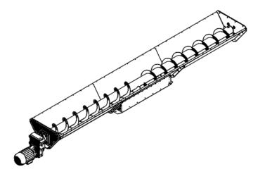
Example: screw conveyor 141.73 in (3600 mm) with outlet on the middle
